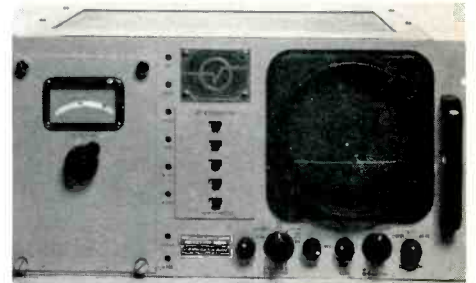
Fig. 3. Nems-Clarke Model SDU-520 combination receiver/spectrum display unit.
