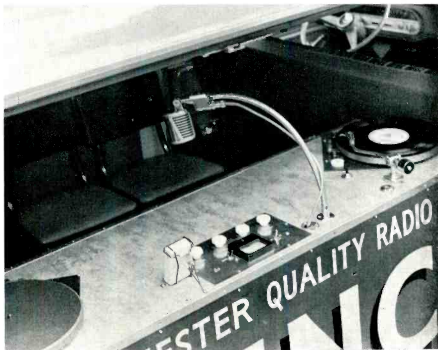
Fig. 2. Transistorized mixer is mounted flush in top of operating table.
