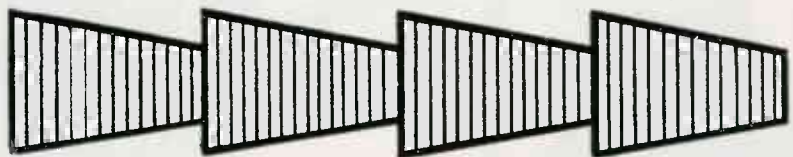
Figure 23 "Slanted" rf envelope of channels at the switcher output usually indicate magnetic video heads.
