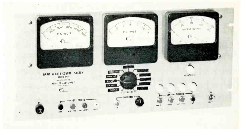
Figure 2. This shows the Studio Control Unit of a radio remote control system. Control signals and metering detection are incorporated in this unit.
