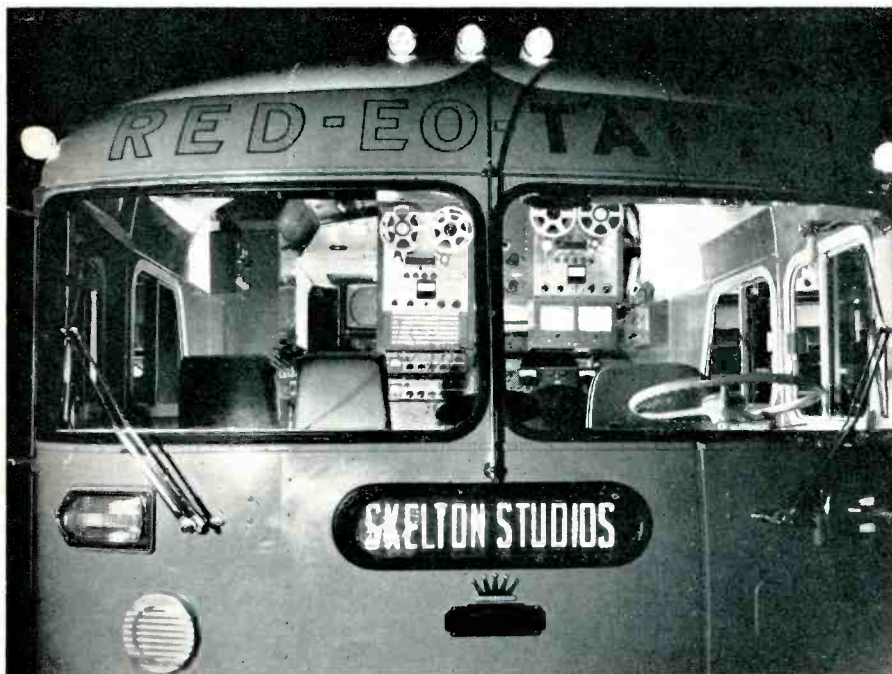
Figure 1. View through the windshield of the control room unit. Visible are two Ampex audio tape recorders which will provide special sound effects for Skelton's Red-Eo-Tape television productions.
