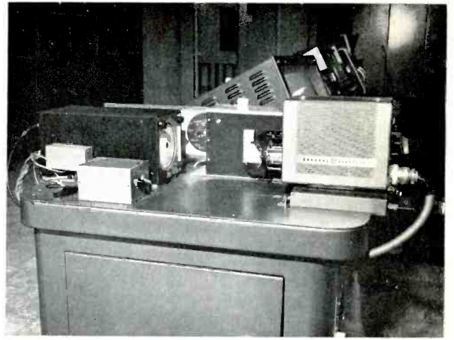
Figure 3. KRLD-TV in Dallas has their radar indicator and vidicon camera installed in the transmitter master control.
