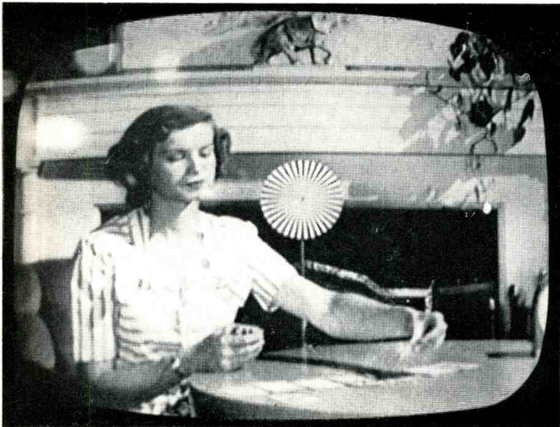
Figure 9. Same image with skew-plate in place. Scratches on the film are optically minimized.
