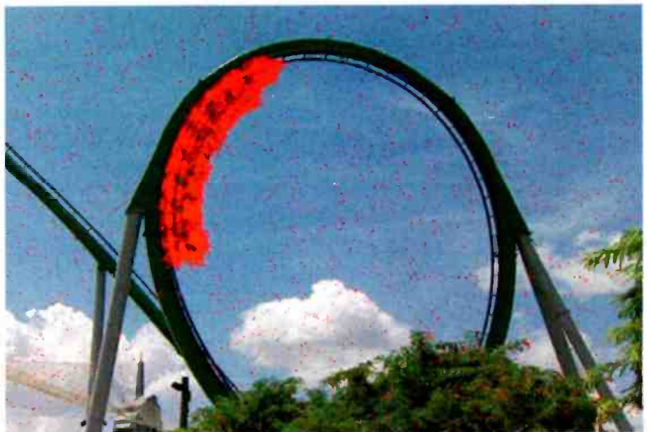
Figure 2. Teranex 2D's display mode presents moving pixels as red pixels.
