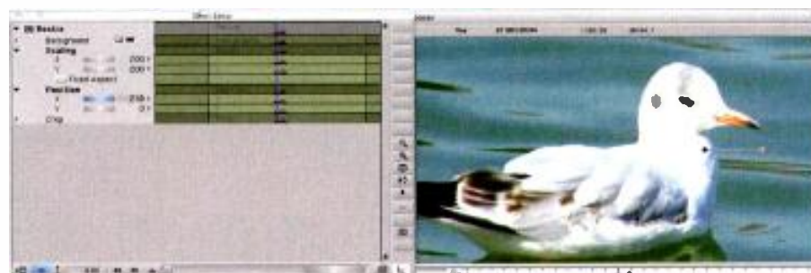
Figure 5. Scaling at 200 x 200 places a 1920 x 1080 window in a 3840 x 2160 frame.
