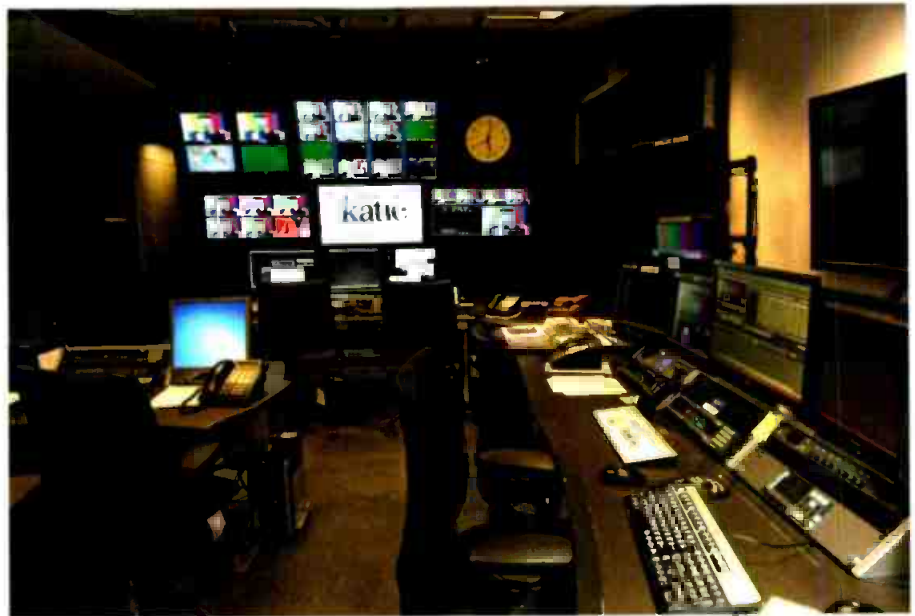
The design team set aside a space within the former TV-1 control room for use as a media center. The media center is built around an EVS server system, and is responsible for the integration of national commercials.
