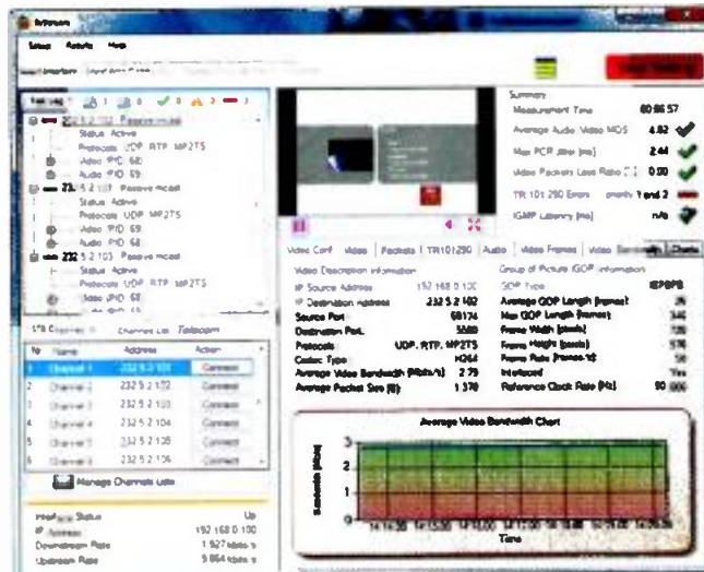
Figure 1. Products such as Fredrick Engineering's feStream provide monitoring and analysis of not only IP network data, but packetized video and audio data as well.
