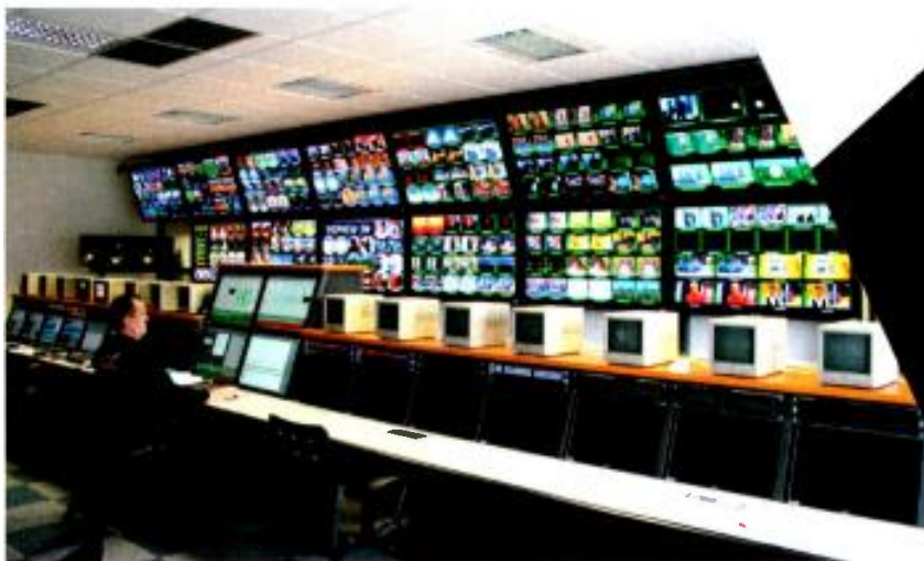
Shown here is multichannel playout monitoring using Miranda's Kaleido multiviewer system at Slovenia-based Satellite Telecommunications Network (STN), a provider of playout and transmission services in Eastern Europe.
