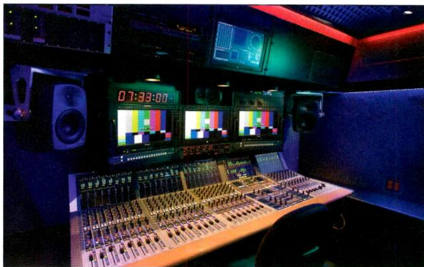
This Touring Video entertainment truck features a Stagetec 32-fader, 110-channel CRESCENDO digital audio mixing console.
