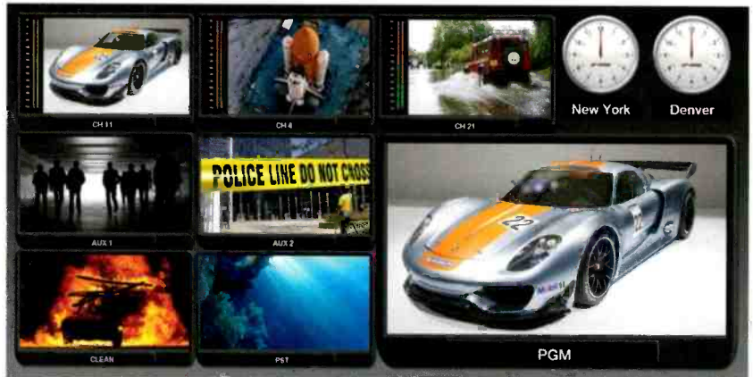
The multiviewer today has evolved into a platform that comes in varying sizes and capabilities, from simple quad-split systems to large-scale, full-facility systems that consolidate routing and monitoring functions.
