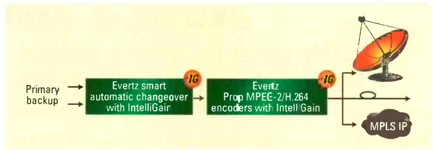
Figure 2. The most common location for audio loudness control is at the transmission stage.
