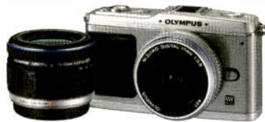
The subject of the article, the tiny 4.8in x 2.8in x 1.4in camera that was used to capture video sequences for large-screen display
