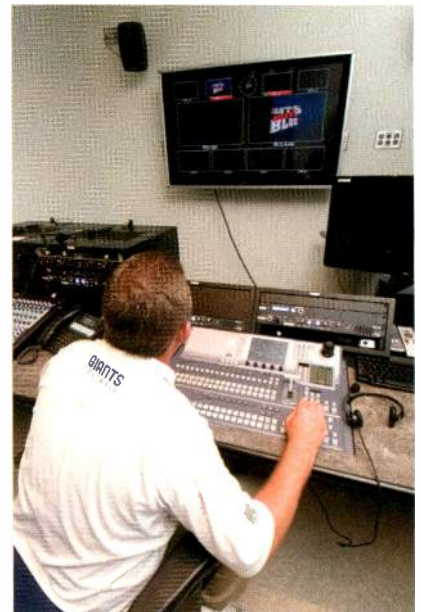
The HD control room at the New York Giants' Meadowlands Sports Complex employs Sony HDC-1400 studio cameras and XDCAM HD optical camcorders, an MFS-2000 production switcher, HDCAM decks, and LUMA LCD monitors.
