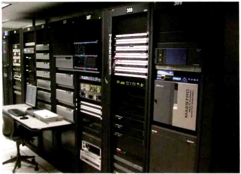
The master control suite houses two Grass Valley Maestro panels with internal branding, DVE, CG, EAS and audio store capabilities; all are controlled by an Avid Sundance Fastbreak NXT automation system and several Grass Valley K2 servers.
