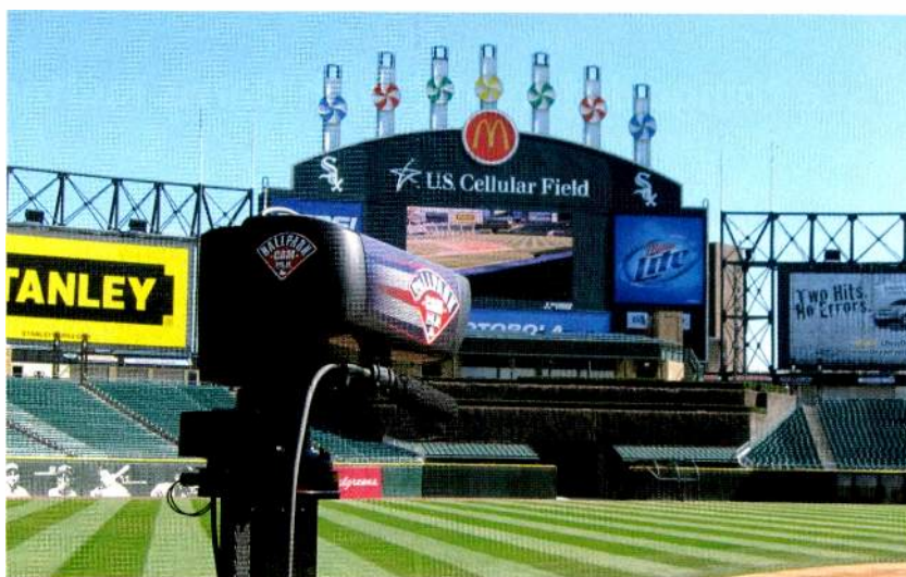
The MLB Network employs a system called BallParkCam. Three signals from up to 15 live games as well as 48 channels of discreet audio are sent live via MPEG-4 4:2:2 AVC encoded streams to the highlights factory, and a clean version is recorded on a local server.
