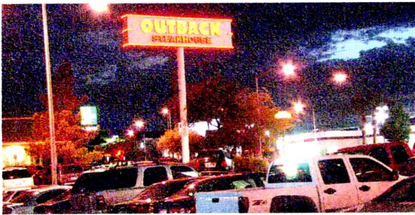
Figure 10. This image was shot with a Sony HVR-V1 using its +36dB hyper gain option. Note the increased noise.
