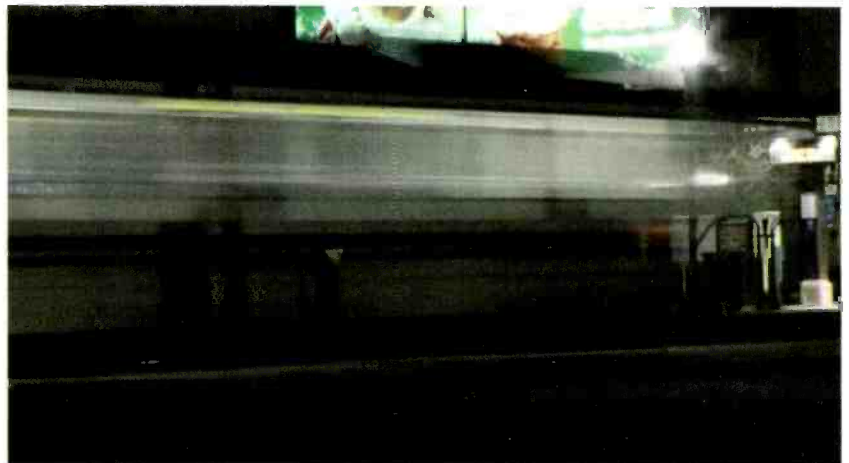
Figure 9. Frame accumulation defines total photodiode integration time as a multiple of the current interframe interval. This image was shot using 16-frame accumulation.
