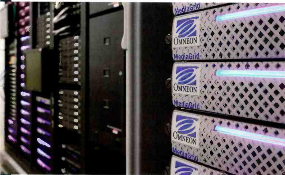
NBC's highly successful Olympic coverage was supported by Omneon's MediaGrid servers in both Beijing and New York. The servers were connected to an Omneon ProCast CDN transport system, which allowed the network to create a U.S.- based, fully interactive, edit-by-proxy content creation system — a 6000mi file-based workflow.
