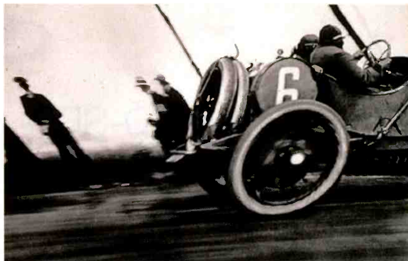
Figure 4. Rolling shutter artifact. This photograph by Henri Lartigue shows a race car skewed in one direction while spectators and telephone poles are skewed in the opposite direction. Lartigue was panning in the direction the car was traveling.
