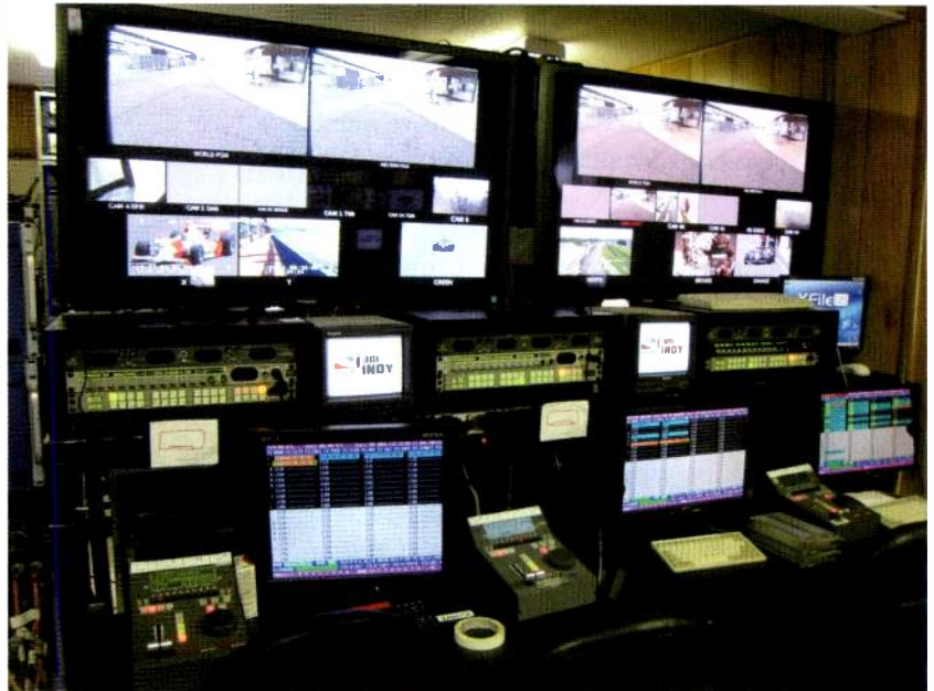
The Kaleido-X supports multiroom display, which was used to drive displays in the world feed EVS room adjacent to the production control room.
