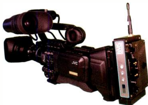
New technology allows crews to venture farther from the ENG truck. For example, the JVC ProHD Libre camcorder has an onboard camera-back transmitter developed by Broadcast Microwave Systems.
