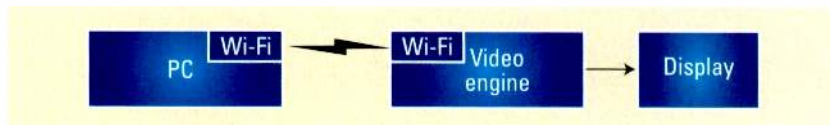
Figure 1. Wi-Fi can relay video, supplied by a PC, to a remote display.
