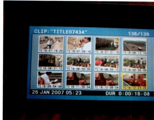
The Sony XDCAM menu system has a logical arrangement. It uses a series of thumbnails to facilitate navigation and review of clips.
