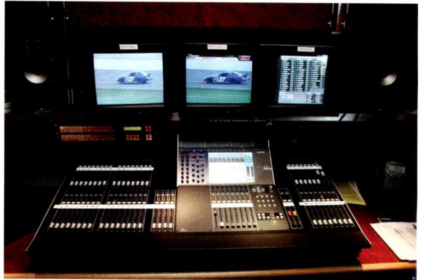
In one of Game Creek Video's trucks for FOX Sports' broadcast of the NASCAR Nextel Cup racing series, this Yamaha M7CL is used for the "Racer Radios" submix. Photos courtesy Jason Taubman, Game Creek Video.
