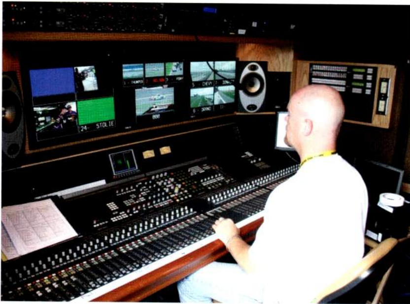
The Calrec Sigma shown here is being used for the track effects audio submix for FOX Sports' broadcast of the NASCAR Nextel Cup racing series.
