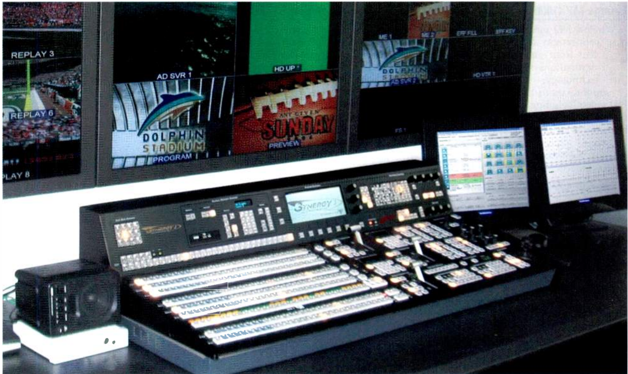
The Miami Dolphins stadium control room uses a Ross Synergy 3 MD-X switcher when broadcasting events such as Miami Dolphins football, Florida Marlins baseball and the FedEx Orange Bowl. The switcher supports all popular SD and HD formats and offers control over VTRs, video servers, audio servers, audio mixers, robotic cameras, routing systems, and more.
