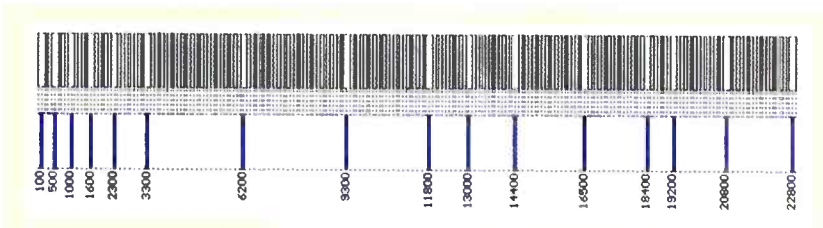
Figure 6. The blue lines indicate the frequencies that can be used free of intermodulation. The black lines indicate intermodulation products.
