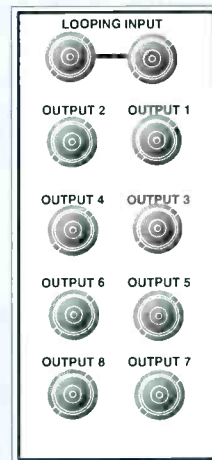
VCA6800+ Double-Slot Back Connector
