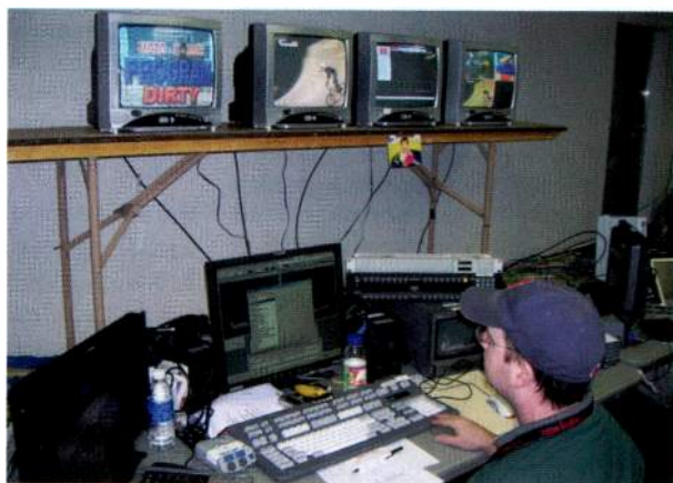
The Deko graphics system can accommodate multiple compositions, permitting simultaneous production of specific formats in HD or SD aspect ratios.
