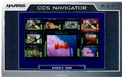
Operators can view up to 32 thumbnails and up to 4 MPEG-4 streams per CCS Navigator™ page
