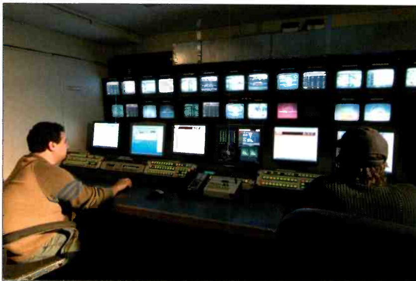
The operators each handle two live program streams sourced from the Omneon servers and real-time races.
