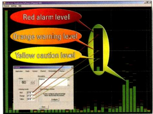
Figure 4. This system's software allows the station to set and adjust alarm points and thresholds.
