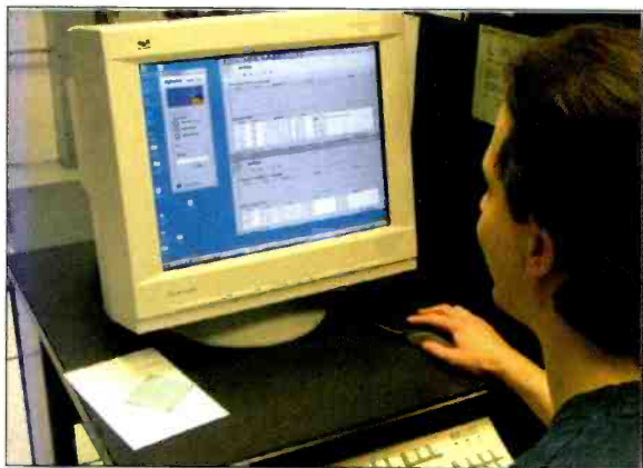
A technician prepares to push commercial spots from the Telestream FlipFactory Traffic Manager server to Lifetime's on-air playback server. This step in the spot-preparation process replaces the need to thread and play a videotape master copy of a commercial.
