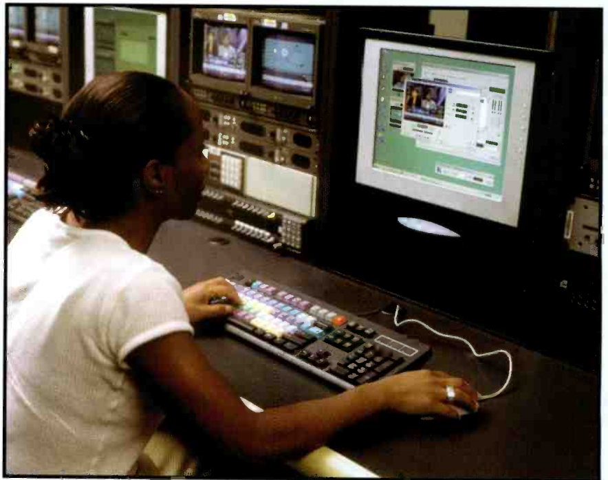
IT-based infrastructure will touch every facet of station operation, including news production. Here one of several Grass Valley NewsEdit systems is used to assemble a story at WJAR-TV in Providence, RI.
