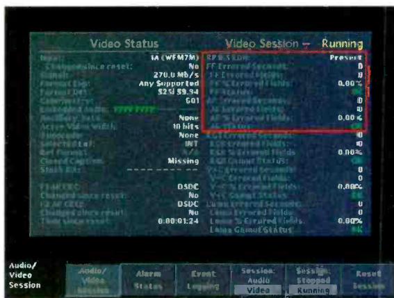
Figure 2. The video-status screen available with various waveform monitors and SDI analyzers can provide status reports of the EDH condition and can log errors.
