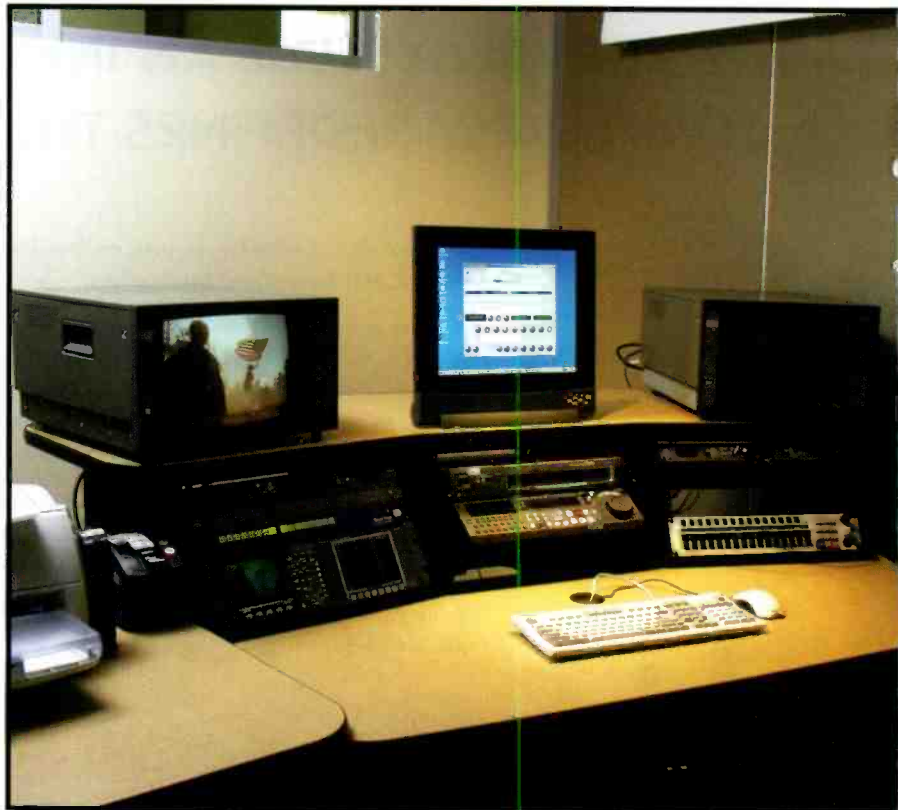
The Turner Cartoon Network uses Snell & Wilcox RollCall terminal technology in the short-form ingest station to centralize control and monitoring functions.
