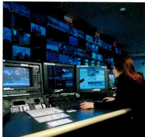
Alex Asaro in the satellite operations center at CNBC, using a custom ILC Maxview control panel and Grass Valley NewsBrowse system to handle dozens of feeds from around the world.
