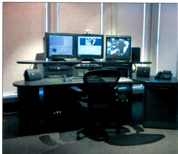
The facility employs an Avid DS system for digital compositing. This system works with the installed Media Composer editing systems and the Unity Media Network to enable staff to perform editing, finishing, audio and graphics work on the same media files at the same time.
