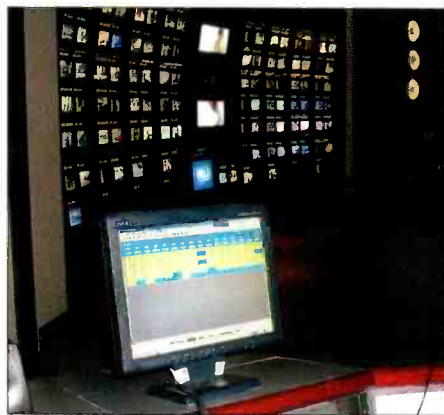
The LABC's control rooms utilize Evertz's VistaLINK to provide operators with a graphical representation of all rooms' monitor walls, enabling a single operator to monitor any room from a single station.
