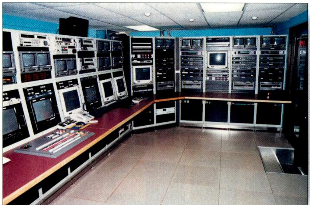
This full view of the Master Control Room at WB-31 shows the Grass Valley Group switcher, the satellite receiver and feed deck.
