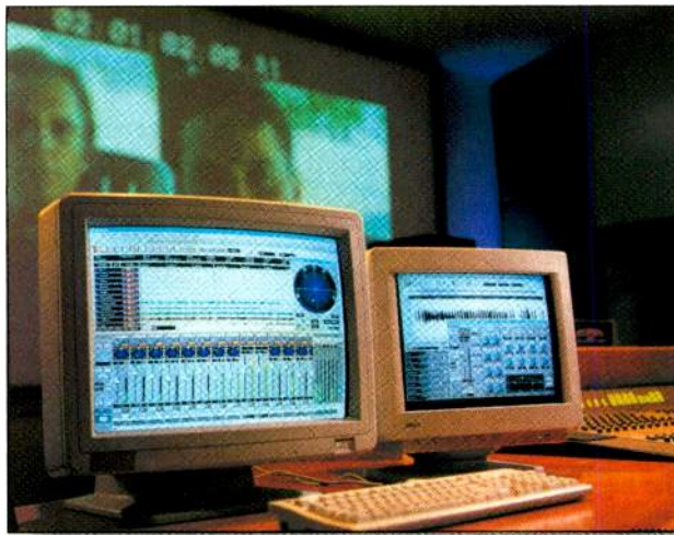
The day of the mixing console may not be past, but control surfaces on workstations like the Nuendo shown above offer users many of the same advantages. Photo courtesy Nuendo.
