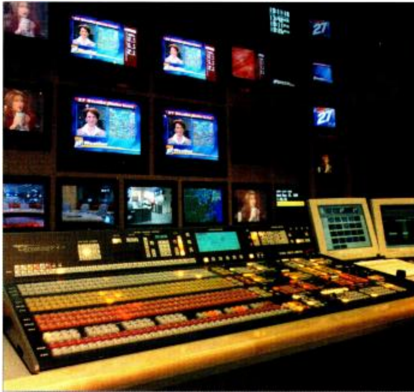
Increasingly sophisticated production capabilities for news and sports, once accomplished with great difficulty on analog production switchers, can be done easily with new digital switching models. Shown here is a Ross Synergy switcher at WKOW in Madison, WI. Photo courtesy of Ross Video.
