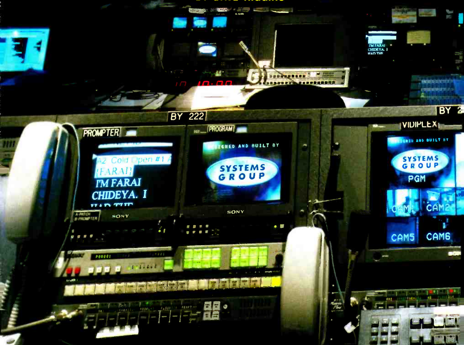
The heavily used Oxygen Production Control Room (Producer's desk in the foreground) also serves as an On-Line Edit Facility. In edit mode, the TD position can operate the entire room. Equipment complement includes Sony DVS 7200 Production Switcher with Shot Box, DME 7000 Core 2 Digital Effects Generator and FX Deko Character Generator. Photos courtesy of The Systems Group. Copyright 2000 Melabee M. Miller.
