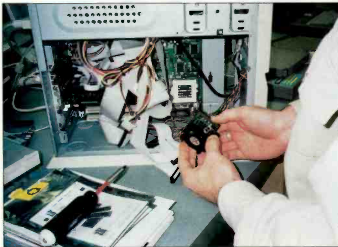
Be sure all the fans are clear of dust.
