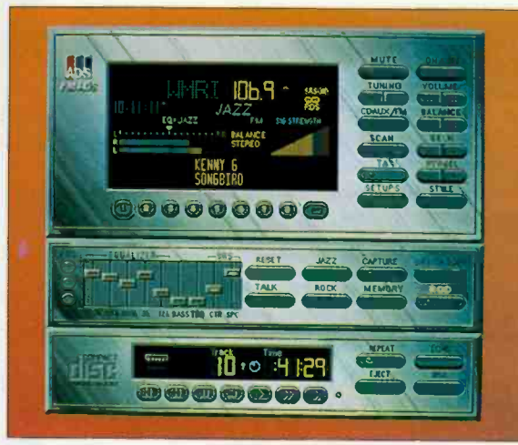
Radio Rock-It from Advanced Digital Systems is a virtual radio for a multimedia PC that uses an FM/RBDS receiver on an internal card with accompanying software to extract RBDS data for the screen display while routing audio to the PC's speakers.
