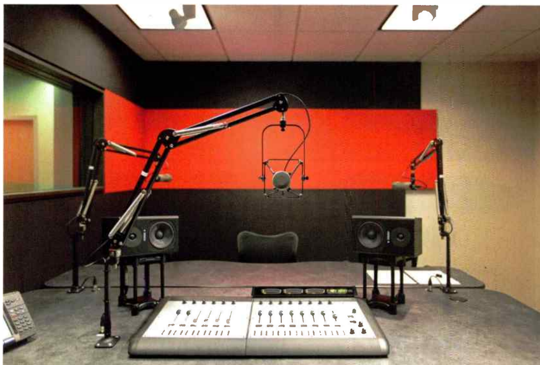
All eight studios feature Axia Radius consoles, with six-fader expansion frames and user keys.
