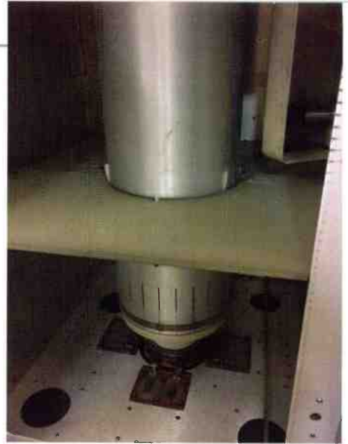
The half-wave cavity lacks the HV blocking capacitor wrapped around the tube anode. However, the high voltage still needs to be kept isolated. Keep all surfaces that isolate DC clean.
