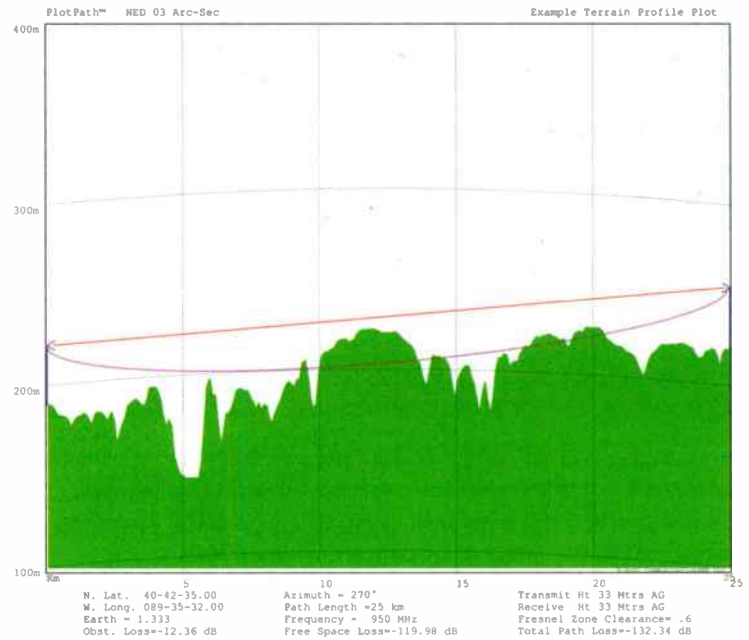
An example of a terrain profile illustrating line-of-sight, but obstruction of the 60 percent of Fresnel zone.
