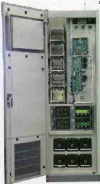
A look inside the V5d with the amplifier modules on the upper left and the power supplies along the bottom.
