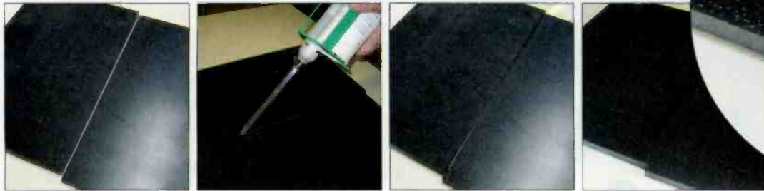
The steps to join solid-surface materials.
