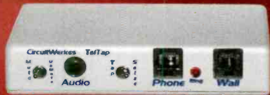
TelTap - Pocket-Sized Manual Telephone Coupler
