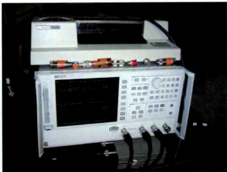
Figure 3. A network analyzer is useful to fully evaluate a transmission line's health.
