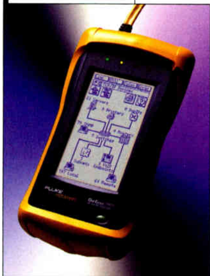
Ethernet testers can evaluate cables, but also provide information on network traffic.
