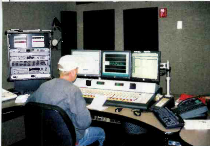
Some studios, like the WOFX control room, have Airwave consoles that will be replaced by RMXdigital consoles next month.
