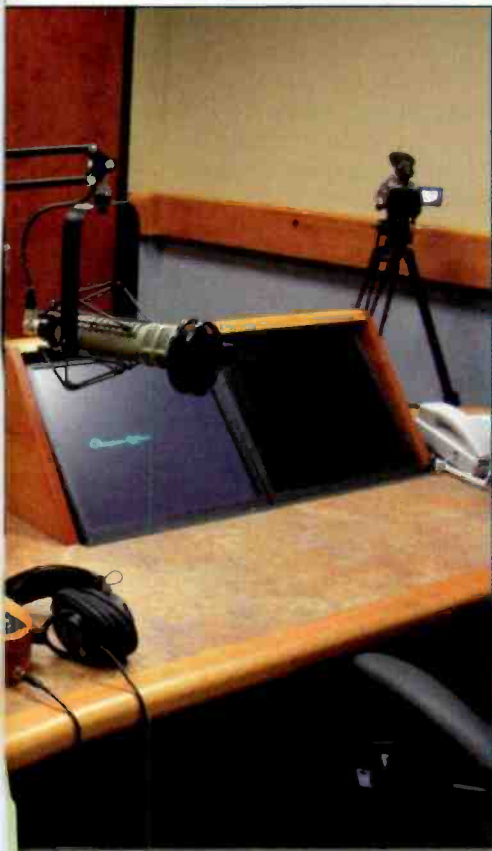
Constructed from Lyptus hardwood, a hybrid hardwood species, the talk studio furniture maintains low sight lines for a clean layout.
