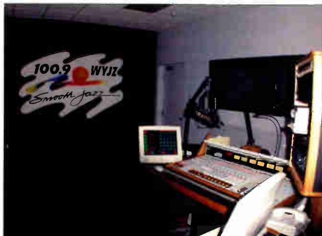
Acoustical foam wedges were hand cut into the shape and design of each station's logo, creating a background for in-studio pictures with on-air personalities.
