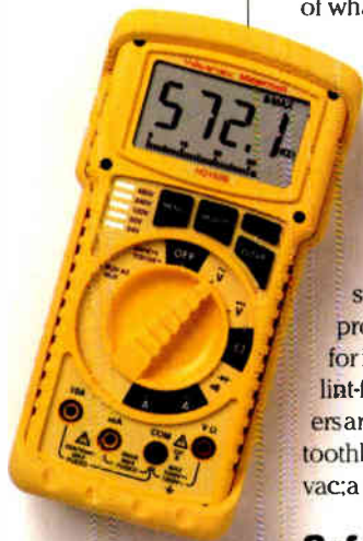
A reliable DMM with appropriate test leads and spare batteries should be kept at a transmitter site.
