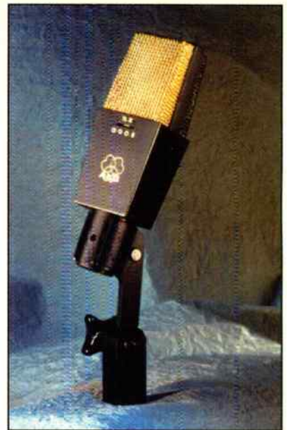
The AKG C414B has a four-position switchable polar pattern.
