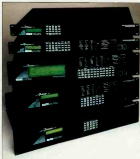
For increased transmission bandwidth, some codecs can bond multiple ISDN lines together.
