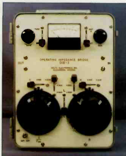
An operating impedance bridge like the OIB-3 from Delta Electronics is invaluable in adjusting antenna networks.
