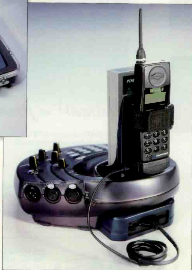
The latest generation of codecs have multiple personalities for use with POTS, ISDN and wireless services.
