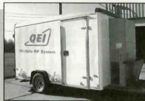
Transportable Pre-Built Transmitter Sites
