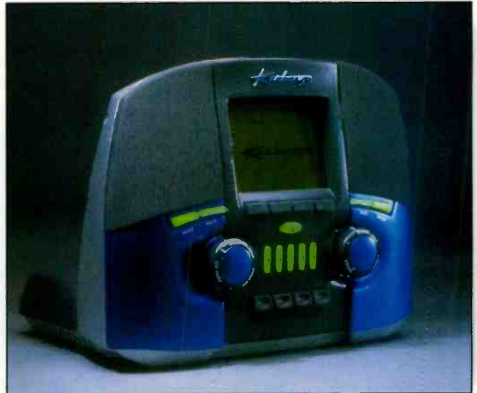
Besides conventional AM and FM signals, the Kerbango tuner receives webcasts.
