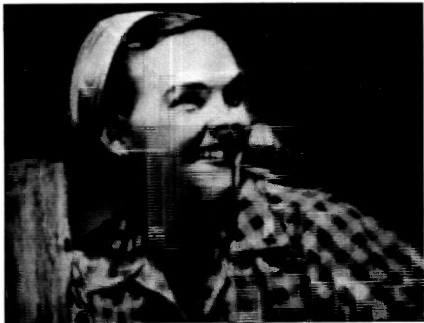
Fig. 3—Reduction of transmission error propagation using predictor output leak ( \alpha = 1/16 , \eta = 128 , 10^{-4} bit error probability).
