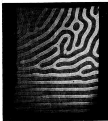
Fig. 4—Faraday observation of magnetic domains in TmFeO_3 . Note the isolated oval domain.
