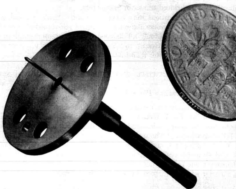
Fig. 6—Example of one of the 0.054" bore coaxial reflection standards used in characterization of transistor jig and bias fixture.
