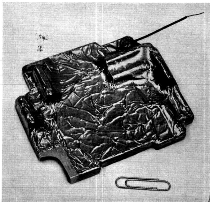
Fig. 10 — Electrostatic shield to isolate subassemblies of modem.
