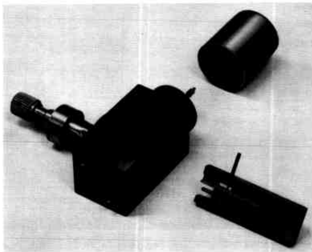
Fig. 1 — Millimeter-wave point-contact wafer diode and holder for use in the 90- to 140-kmc frequency band.
