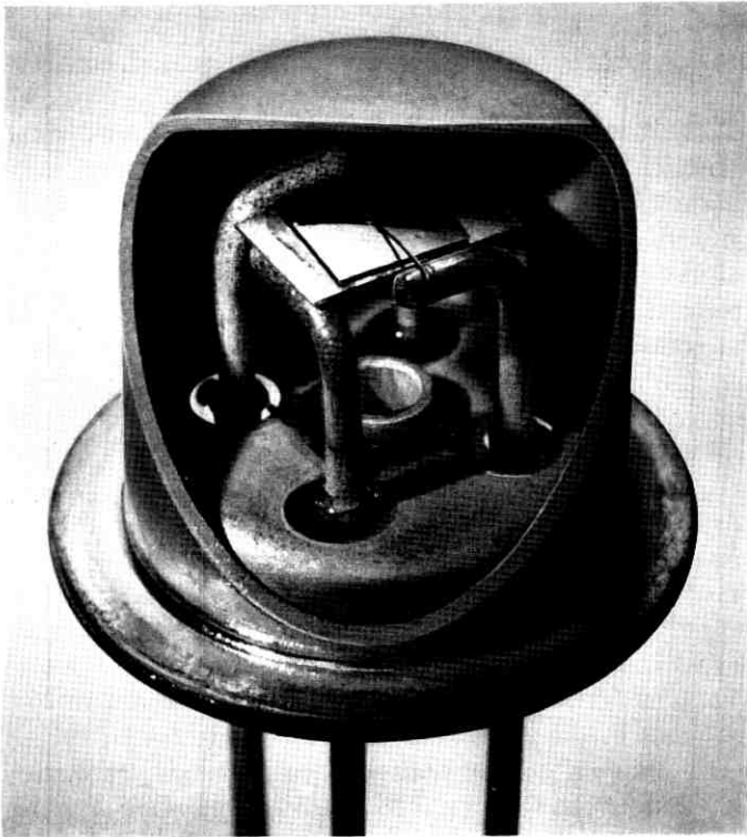
Fig. 6 — Construction of the radiation damage transistors.
