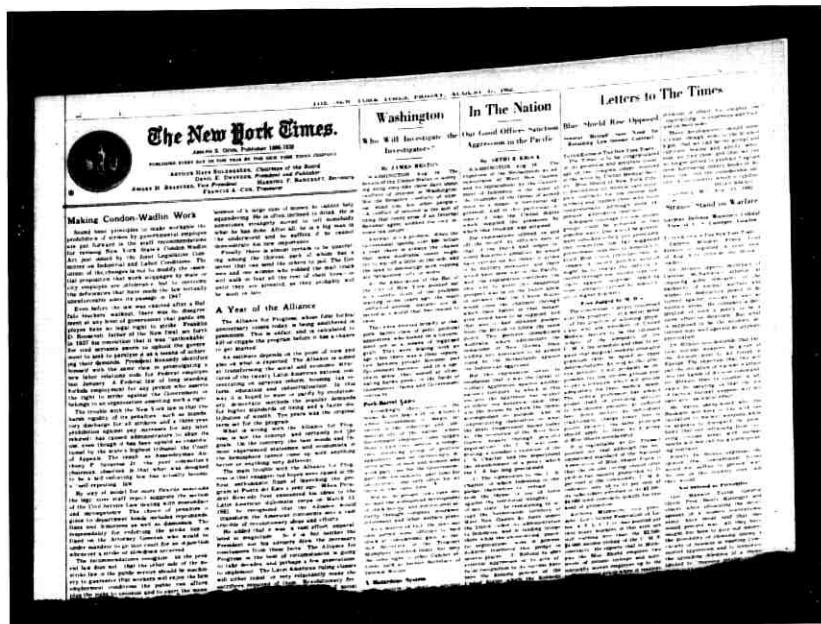
Fig. 51 — High-speed, two-tone facsimile; satellite loop, pass 352. (Frame skew is due to changing absolute time delay for the synchronizing signal.)
