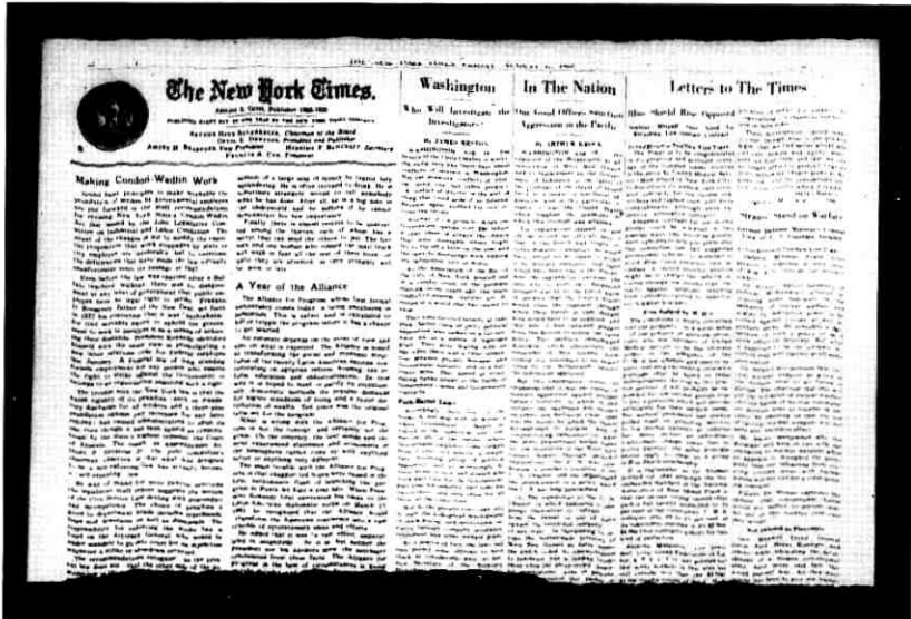
Fig. 50 — High-speed, two-tone facsimile; satellite loop, pass 352, Aug. 17, 1962. (Keying rate is 675 kc. Jitter is due to unfiltered transients in the landline facilities.)
