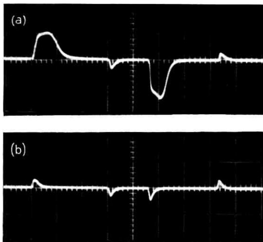
Fig. 15 — (a) Output waveform obtained by nondestructive interrogation of a core containing a one. (b) Output waveform obtained when the core contained a zero. Vertical calibration = 0.1 volt per division; horizontal calibration = 2 \mu\text{s} per division.
