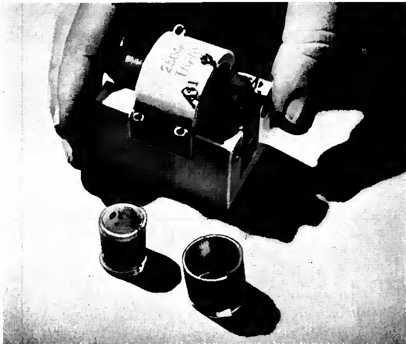
Fig. 3 — Transformer and separate inner and outer winding forms with windings.
