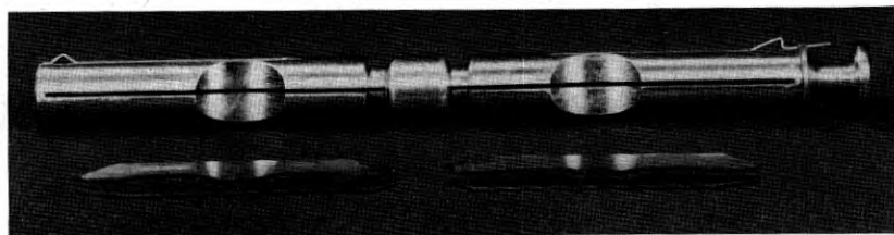
Fig. 6 — Double spindle showing slots and complement of two sets of die blades.
