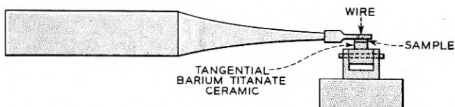
Fig. 7—Experimental arrangement for studying frictional forces.
