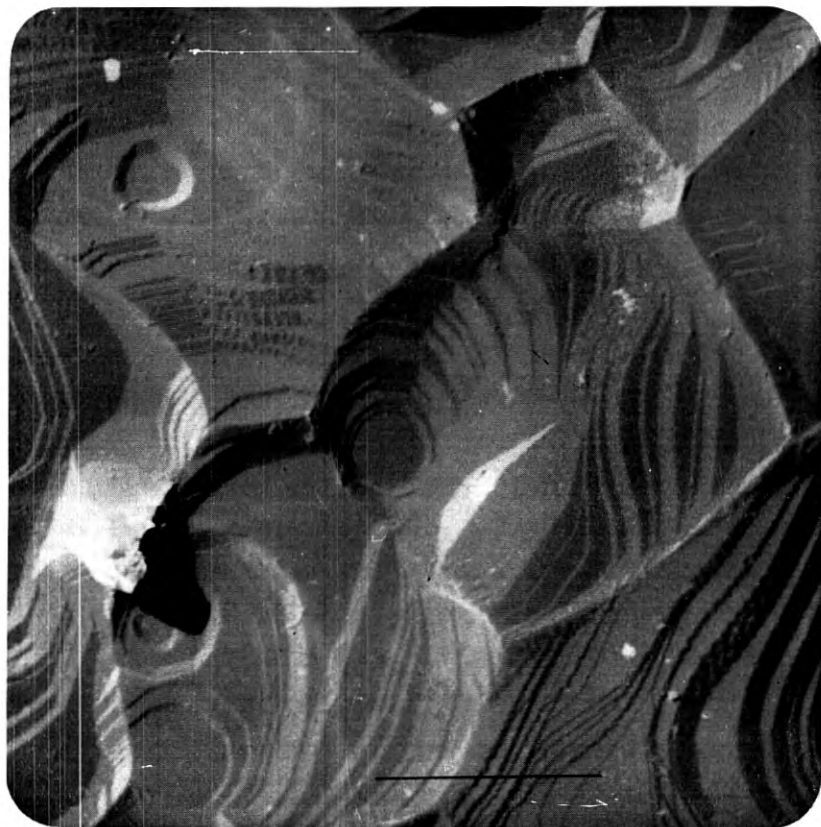
Fig. 14—Germanium replica ( t_e \simeq 150\text{\AA} , \theta_a = 35^\circ ) of near optimum thickness. Resolution about 75\text{\AA} . Ruptured film evident in shadow.
